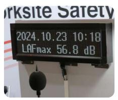
**Public Sound Level Displays:** Connects to LED signage, allowing everyone to easily notice when noise levels exceeded.
